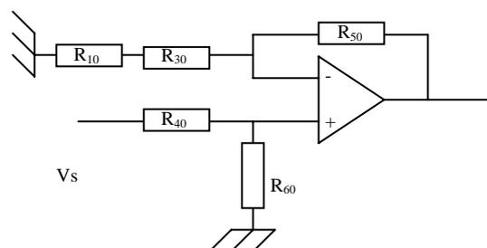
$$V_+ = \frac{R_{60}}{R_{40} + R_{60}} V_2$$
